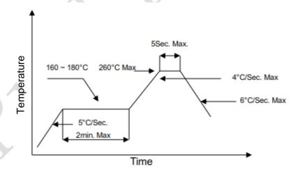
Note: Reflow soldering can be operated only one time. During the temperature ramp-up, no forces may be exerted on the VP which could deform or damage them. After soldering completed, please also do not process until the product temperature ramp down to room temperature.
