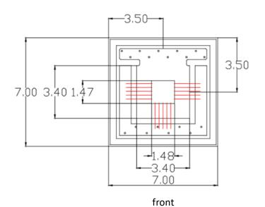
VD-0940I-004W-1K-2A0 with Substrate 1=<u>AIN</u> and Package K=<u>T-mount</u> (unit: mm)
