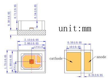
VD-0940C-060M-3A-2A0 (Substrate CuAg, 2016 packaging, unit: mm)
