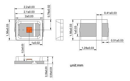
VD-0940C-060M -3E-2A0 (substrate Cu/Ag, 7060 packaging), unit:mm
