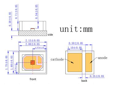
VD-0940C-008M-XX-2A0 with Substrate 3=<u>Cu/Ag</u> and Package I=<u>To46</u> (unit: mm)
