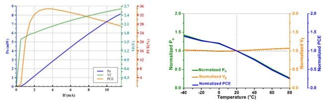
**Note:** 1. LIV graph was measured at 25 °C (left); power output, voltage and power conversion efficiency variation trend with changed operating temperature (right, normalized).
