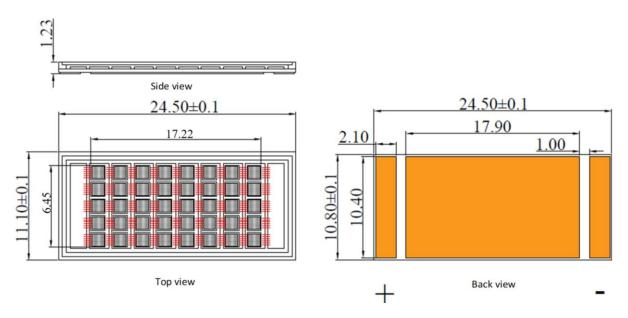
VD-0940I-100W-6K-3A0 with Substrate 6=Cu and Package T=T-mount (unit: mm)
