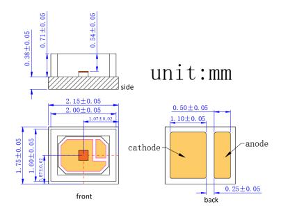
VD-0940V-020M-1C-2B0 with Substrate 1=AIN and Package C=3535 (unit: mm)
