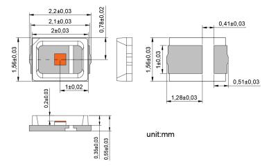
VD-0940V-020M-1A-2B0 with Substrate 1=AIN and Package A=2016 (unit: mm)
