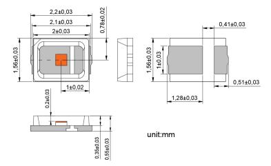
VD-0940V-015M-1A-2B0 with Substrate 1=AIN and Package A=2016 (unit: mm)
