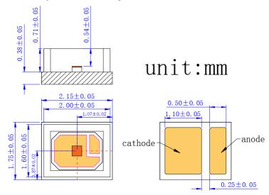
VD-0940I-025W -3A-3A0 (Channel array 1X1, Substrate CuAg, Package 2016)
