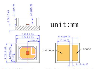
VD-0940I-010W -3A-3A0 (Channel array 1X1, Substrate CuAg, Package 2016)
