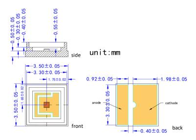
VD-0940I-001W-3E-2A0 with Substrate 3=Cu/Ag and Package E=7060 (unit: mm)
