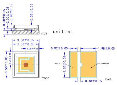
VD-0940C-060M-3C-2A0 with Substrate 3=<u>Cu/Aq</u> and Package C=<u>3535</u> (unit: mm)
