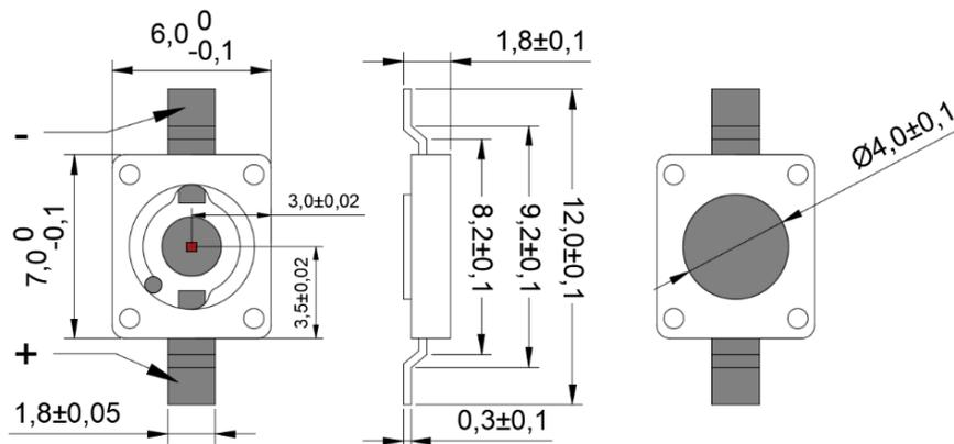
**VD-0850I-700M-1A-3A0 (substrate AlN 2016 packaging), unit:mm**
