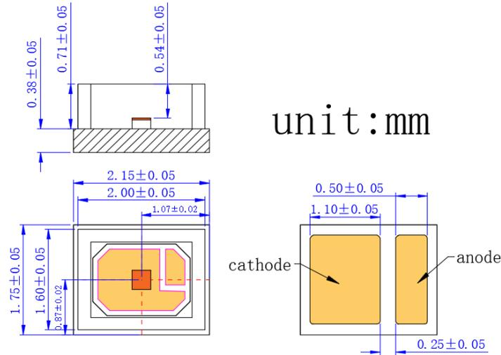
**VD-0850I-700M-1C-3A0 (substrate AlN 3535 packaging), unit:mm**
