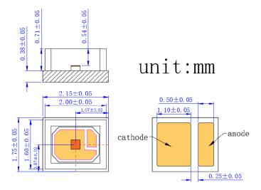
VD-0850I-130M-1C-2A0 with Substrate 1=AIN and Package C=3535 (unit: mm)
