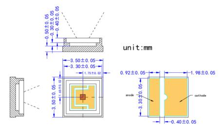
VD-0850I-130M-3A-2A0 with Substrate 3=Cu/Aq and Package A=2016 (unit: mm)
