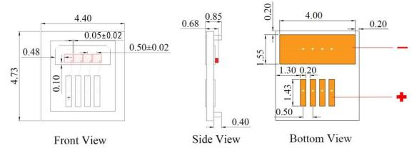
VD-0850I–050W –10–3A0 (Channel array 1x8, Substrate Cu/Ag, Package 1x8)
