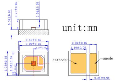
VD-0850I-050W -3A-3A0 (Channel array 1x1, Substrate Cu/Ag, Package 2016)
