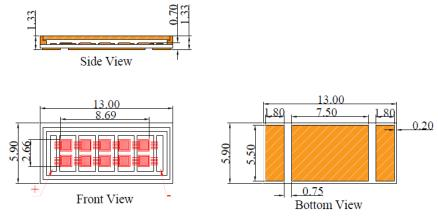
VD-0850I-020W-6K-2A0 with Substrate 6=Cu and Package K=T-mount (unit: mm)
