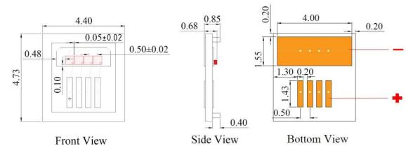
VD-0850I–015W –10–3A0 (Channel array 1x8, Substrate AIN, Package 1x8)
