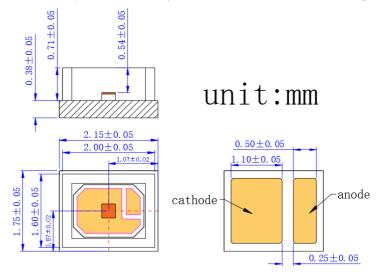
*VD-0850I–015W –3A–3A0* (Channel array 1x1, Substrate CuAg, Package 2016)
