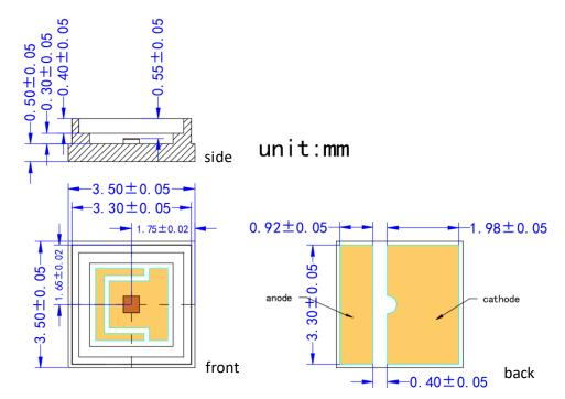
VD-0850I-002W-3E-2A0 with Substrate 3=Cu/Ag and Package E=7060 (unit: mm)
