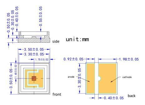
VD-0850I-001W-3E-2A0 with Substrate 3=<u>Cu/Ag</u> and Package E=<u>7060</u> (unit: mm)
