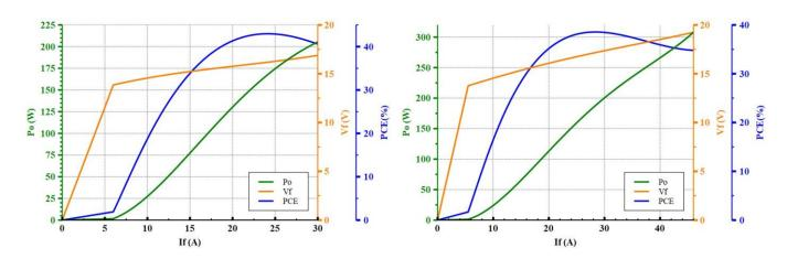
(right): CW mode; (left): Pulse mode at Pulse width 100ms & Duty cycle 10%.
