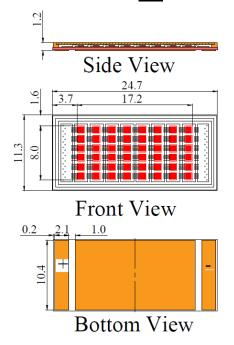
VD-0808I-220W-1U-2A0+Case (Substrate 1=AIN and Package U=2511, with water cooled case (unit: mm)
