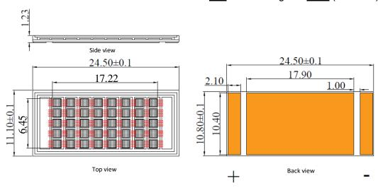
**Note:** Soldering procedure: The base plate is at right angles, and there is no bevel or chamfer. The copper clad and the substrate copper cannot be layered for 30 minutes at 300 degrees
