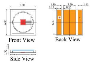
VD-0808I-007W-6K-2A0 with Substrate 6=Cu and Package K=T-mount (unit: mm)
