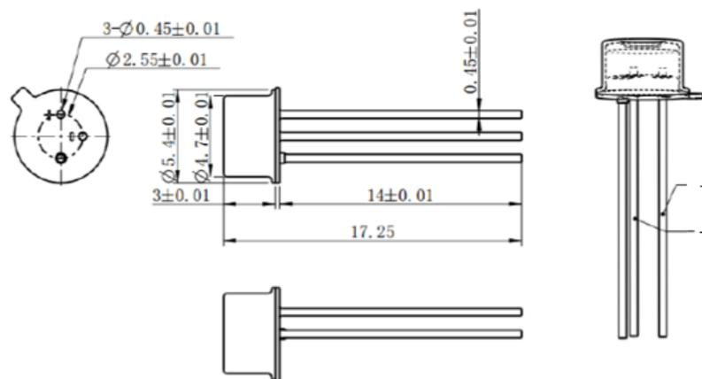
VD-0940C-008M-XX-2A0 with Substrate 3=CuAg and Package A=2016 (unit: mm)
